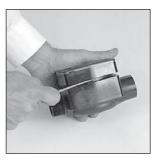
Remove the signal generator from the pin on the nutator disc. (Figure 5)
