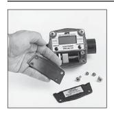
3. Remove the battery and, if necessary, clean corrosion from the battery terminals. (Figure 9) To prevent corrosion from condensation, coat the terminals with petroleum jelly.
