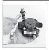
Gently pry the coverplate from the housing. Take care not to damage the coverplate, housing, or O-ring. (Figure 4)
