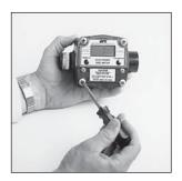
2. Remove the battery coverplate and gasket. (Figure 8)
