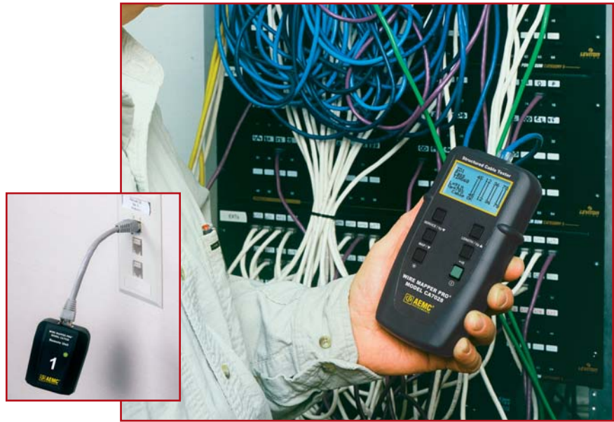
Model CA7028 used to locate and test a cable from the patch panel to an office a few hundred feet away.
