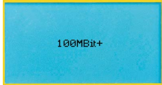
Service test function determines speed and type of transmission.
