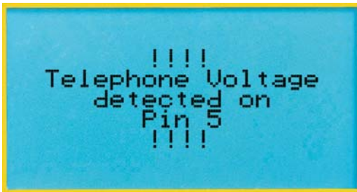
Automatic detection of live telephone voltage.
