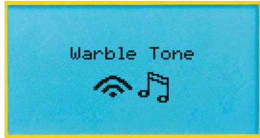
Built-in tone generator for cable tracing.
