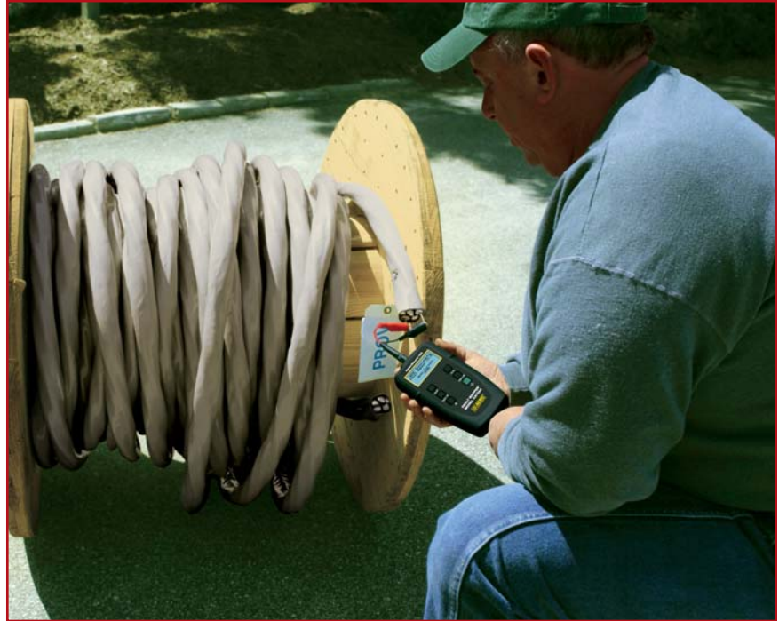
Model CA7024 checking the length of power cable on a reel.
