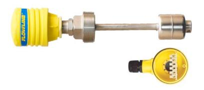
The general purpose float level transmitter provides continuous level measurement up to 6.5' (2m) with a 4-20 mA signal output, and is factory configured to your selected dimension. This stainless steel liquid level sensor is well suited for high temperature or pressure tank level applications with relatively clean liquids such as water, diluted chemicals and light weight oils. Application examples include boilers and process vessels.
