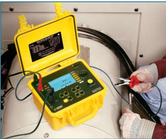
Model 5060 performing insulation test on a generator.
