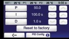
The Performance Programmable Controller's performance is easily fine tuned by selecting a specific heat transfer fluid, entering a fluid's specific heat capacity value, or even adjusting PID settings.
