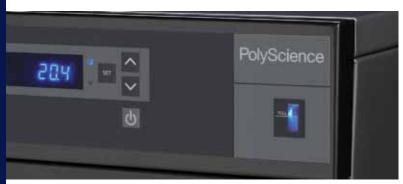
Front mounted fluid level gauge lets you quickly determine if coolant needs to be added to the reservoir.
