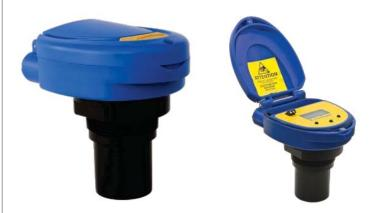
The general purpose ultrasonic level transmitter provides continuous level measurement up to 32.8' (10m) with a 4-20 mA signal output, and is configured via its integral push button display module. This noncontact liquid level sensor is ideally suited for corrosive, ultrapure, sticky or dirty liquids, and is broadly selected for bulk storage, day tank, lift station and process tank level applications.
