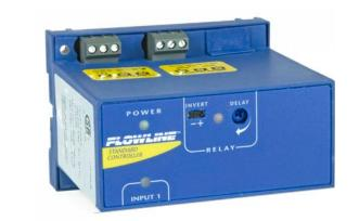
The general purpose flow controller is offered in two configurations for low-flow pump and process protection. The LC80 accepts one flow sensor input and provides one 10A relay for low flow control. The LC82 accepts two flow sensor inputs and provides two 10A relays for dual low flow control. Package this flow controller with our liquid or gas flow switch sensors. For field mount installation, add a single or dual controller NEMA box.
