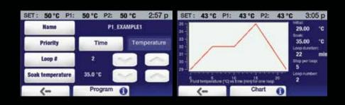
Special features, such as the ability to select time or temperature as the priority and preview the resulting temperature profile, eliminate the guesswork when creating time/temperature programs.
