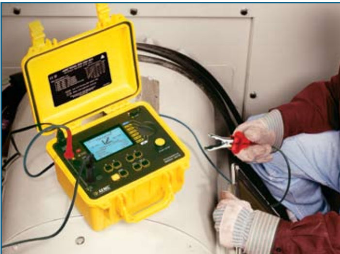
Model 5070 performing insulation test on a generator.
